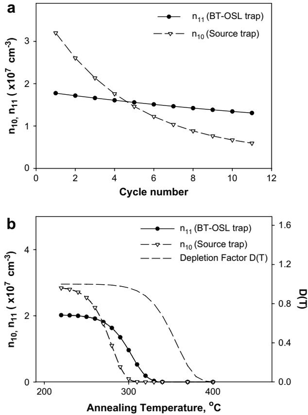
**Fig. 2.** (a) The simulated temperature dependence of the charge concentrations in the source traps ( $n_{10}$ ), and the BT-OSL traps ( $n_{11}$ ), during the repeated cycles experiment of Wang et al. (2006b). (b) Same as (a), for the annealing experiment of Wang et al. (2006b). The slightly modified parameters of Table 1 are used in both simulations shown in (a) and (b).
