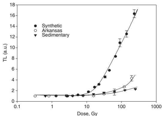
Figure 2. The sensitivity of the ‘110°C’ glow-peak as a function of the predose only, normalised to the sensitivity at the lowest predose.
