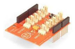
Open your TINKERKIT box, and remove gently the ARDUINO SHIELD. Place the shield on top of the Arduino board and align ALL the pins.
