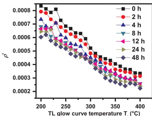
Fig. 7. The dependence of the dimensionless parameter  $\rho'$  evaluated from the fitting procedure using Eq. (2), on the glow-curve temperature for various grain sizes.
