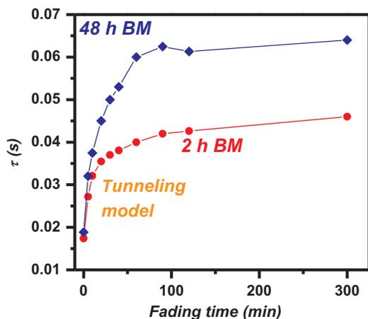
Fig. 10. The behavior of the mean tunneling recombination lifetime for the unique component of the OSL signal, for ball milling durations of 2 and 48 h, as a function of storage time. The behavior of all other grain sizes is between that of 2 and 48 h BM.
