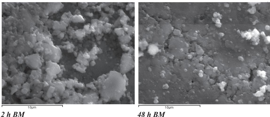
Fig. 1. SEM backscattered images of ball milled Durango apatite after 2 h (left) and 48 h (right) ball milling.
