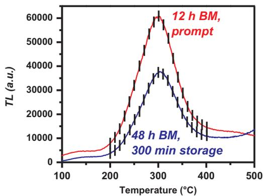
Fig. 6. TL glow-curves of Durango apatite for (a) prompt measurement after 12 h BM and (b) for storage time of 300 min corresponding to 48 h BM. The vertical bars on the glow curves show the temperatures  $T_i$  from which TL integrations over  $10^\circ\text{C}$  occur, to evaluate the AF rate as a function of the glow curve temperature.
