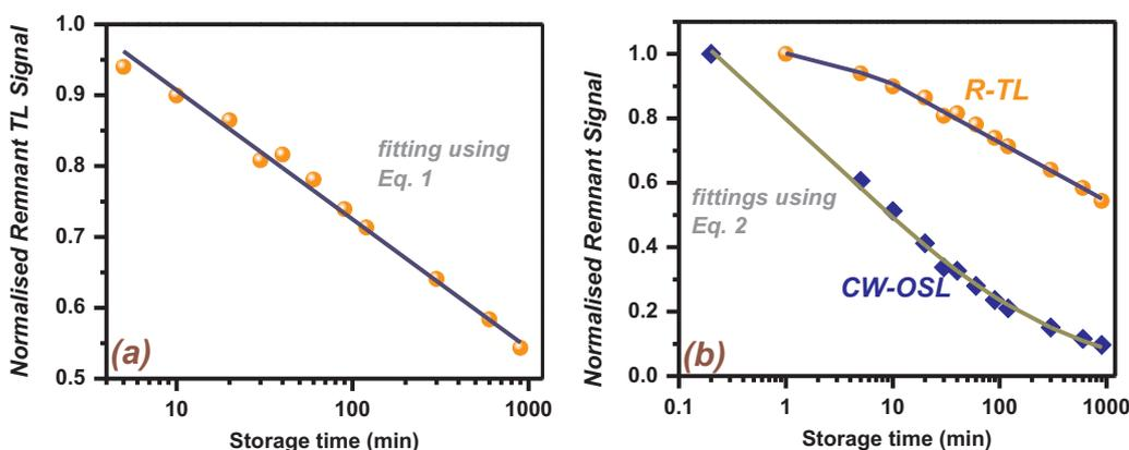
Fig. 4. Fitting examples of (a) normalized R-TL as a function of storage time using Eq. (1) and (b) normalized R-TL and residual OSL as a function of storage time using Eq. (2).
