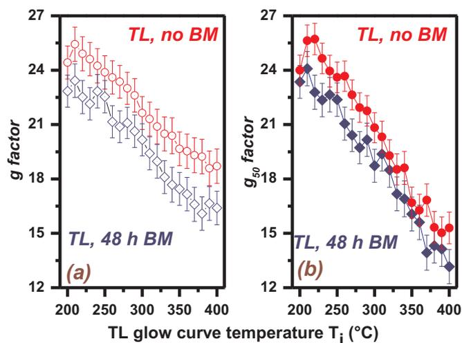
Fig. 8. Plot (a) depicts the values of the  $g$ -factor evaluated from the fitting according to Eq. (1), as a function of the glow-curve temperature for ball milling durations 0 and 48 h. Plot (b) presents the values of the  $g_{50}$  factors, evaluated from the  $\rho'$  values of Fig. 7 using Eq. (3) for ball milling durations 0 and 48 h versus the glow curve temperature. The behavior of all other ball milling durations lies between that of 0 and 48 h of BM.
