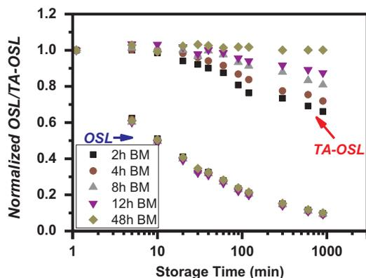
Fig. 3. Normalized residual OSL and TA – OSL output as a function of storage time for various ball milling times.
