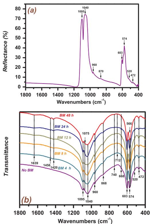
Fig. 12. FTIR spectra of (a) Durango fluorapatite single crystal in reflectance mode and (b) in transmittance mode from the initial grinded material as well as after 4, 8, 12, 24 and 48 h of ball-milling procedure. The wavenumbers of the main bands are also presented in arrows.
