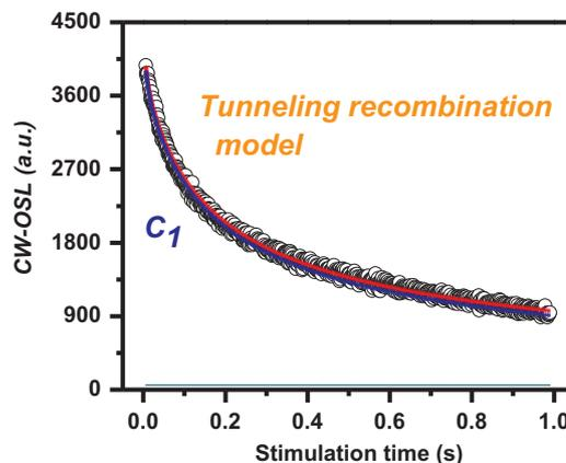
Fig. 9. CW-OSL curve, analyzed using the tunneling recombination expressions according to Eqs. 6 and 7.
