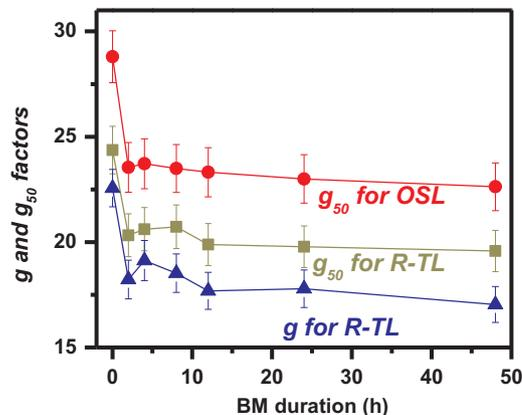
Fig. 5.  $g$  and  $g_{50}$  factors versus BM durations. The  $g$  factors were evaluated according to Eq. (1) using the integrated luminescence intensity; an example of the corresponding analysis is presented in Fig. 4a. The  $g_{50}$  factors were evaluated by using Eq. (3), after evaluating  $\rho'$  according to Eq. (2), using the integrated luminescence intensity; an example of the corresponding analysis is presented in Fig. 4b.
