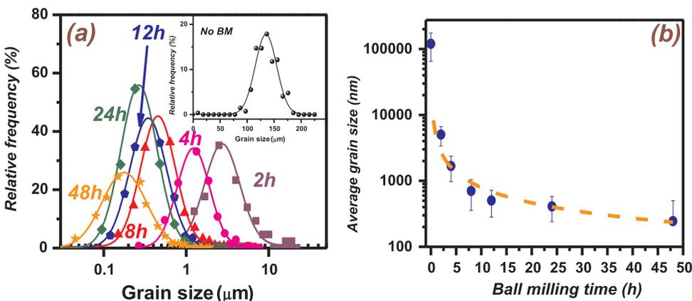
Fig. 2. Plot (a) presents the grain size distribution for different ball milling durations. The inset shows the distribution for the powder without ball milling. Plot (b) presents grain size versus the ball milling duration in terms of the centroid of each distribution presented in plot (a). Errors are expressed as  $1\sigma$ . The dashed line provides a guide for the eye.
