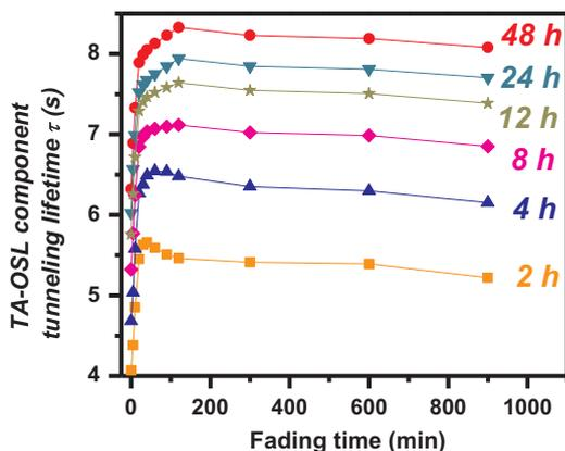
Fig. 11. The behavior of the mean tunneling recombination lifetime of the first component of the TA – OSL for all ball milling durations (2–48 h) as a function of the fading storage time. For the other component of the TA – OSL signal, the OTOR model was used, according to Eqs. 4 and 5; the corresponding lifetime is stable, independent on both ball milling and fading times.
